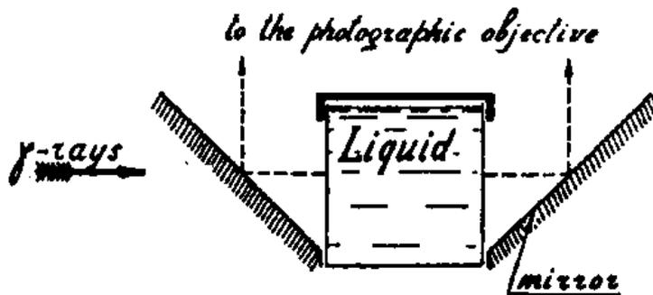
Figure 1: Arrangement of apparatus.
