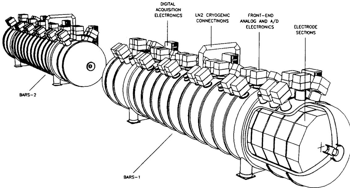
Fig. 4. BARS calorimeters.
