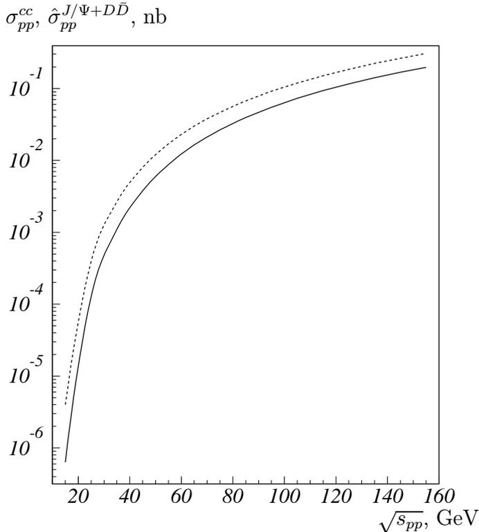
Fig. 5. The total cross-section of the proton-proton production of  $(cc)$ -diquark and  $J/\Psi + D\bar{D}$  (solid and dashed curves, correspondingly).
