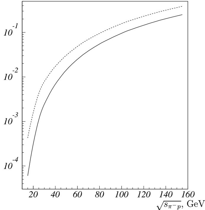
Fig. 4. The total cross-section of the pion-proton production of  $(cc)$ -diquark and  $J/\Psi + D\bar{D}$  (solid and dashed curves, correspondingly).
