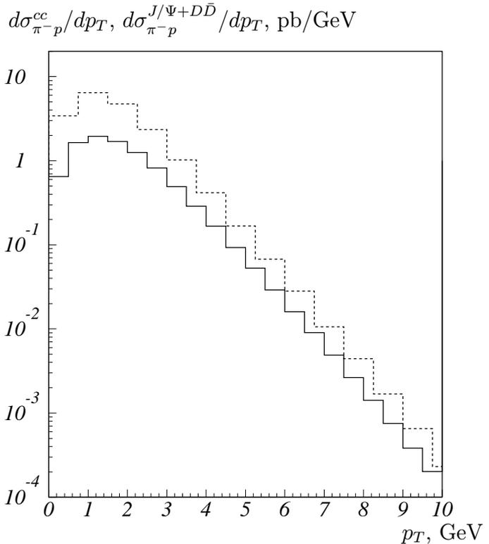
Fig. 6. The  $p_T$ -distributions for the production of doubly charmed diquark (solid histogram) and associated  $J/\psi$  (dashed histogram) at the pion-proton interaction energy of 35 GeV.
