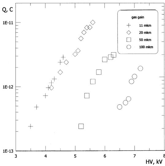
Fig. 3. Gain versus electric field strength for: 11 μm, 20 μm, 50 μm and 100 μm diameter anode wires.
