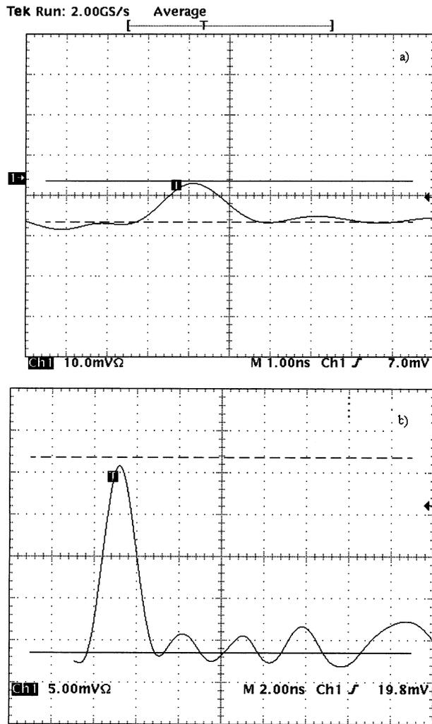
Fig. 2. Average signal waveforms, measured directly on 50Ω inputs of TDS724 oscilloscope: from  $Fe^{55}$ (a) and from  $Sr^{90}$ (b), radioactive sources, correspondingly.
