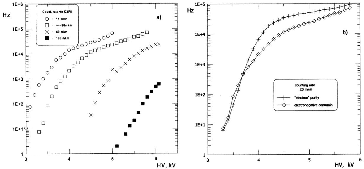
Fig. 1. Counting rates measured a) with “electronically graded” freon - $11\mu\text{m}$ , - $20\mu\text{m}$ , - $50\mu\text{m}$  and - $100\mu\text{m}$  diameter anode wire; b) with “electronical” (...) and commercially available (...) freons, correspondingly.
