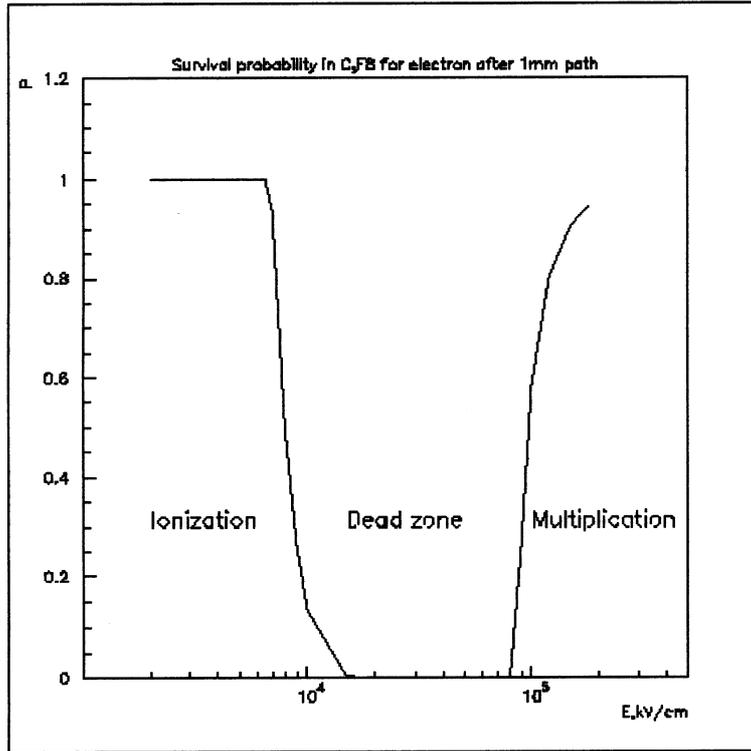
Fig. 6. The survival probability to survive for at least one electron after 1mm path in  $C_3F_8$  at atmospheric pressure as a function of electric field strength.
