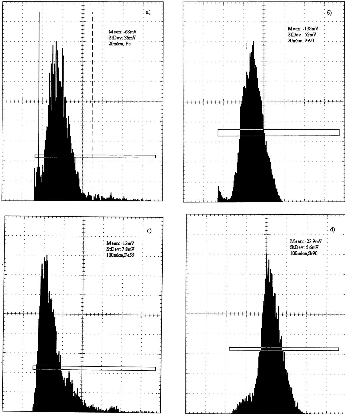
Fig. 5. Pulse height spectra, measured from  $Fe^{55}$  and  $Sr^{90}$  irradiations for 20 $\mu$ m and 100 $\mu$ m anode wires.
