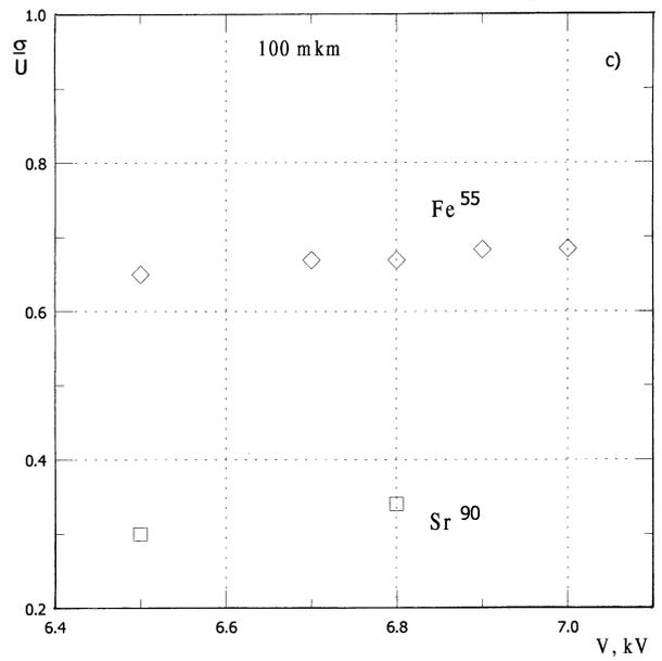
Fig. 4. Relative spectrum widths after  $\text{Fe}^{55}$  and  $\text{Sr}^{90}$  irradiations taken with 20  $\mu\text{m}$  (a), 50  $\mu\text{m}$  (b) and 100  $\mu\text{m}$  (c) anode wire diameter counters, correspondingly.
