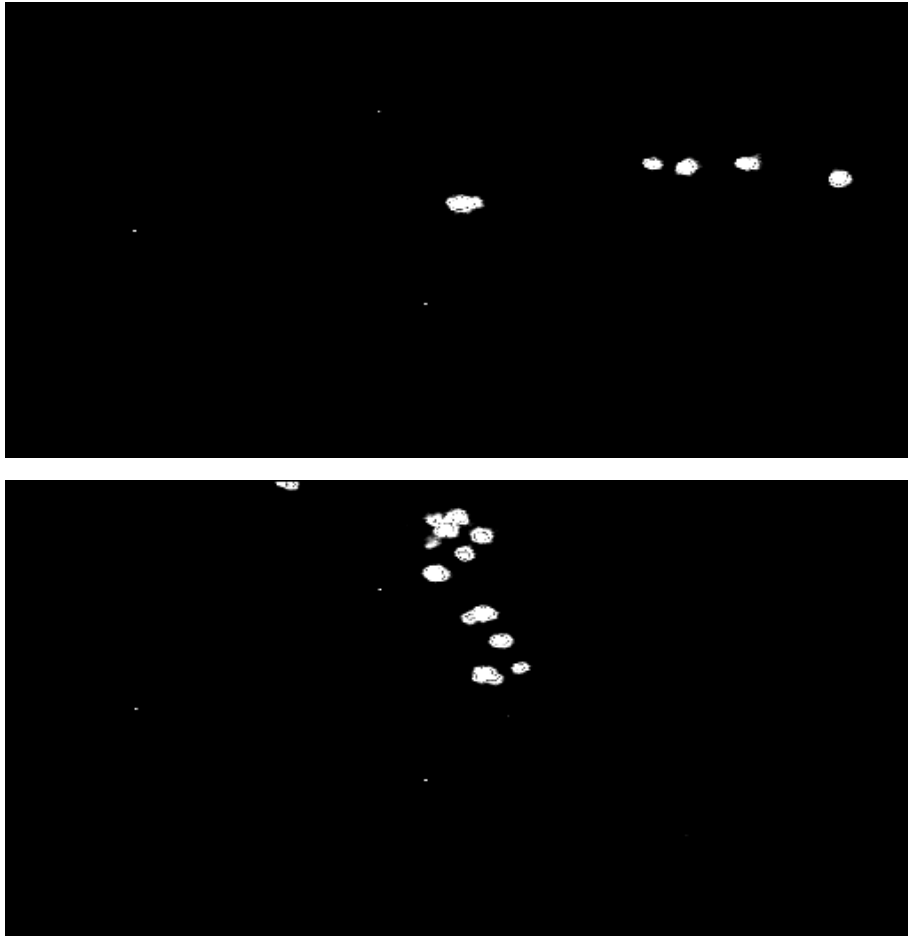
Fig. 11. Two examples of picture obtained with CCD camera for streamer discharge.
