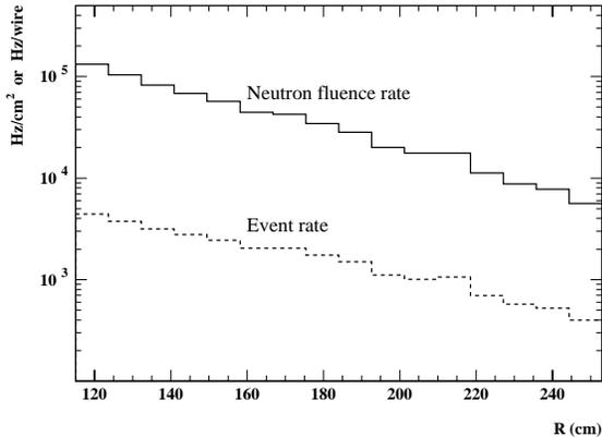
Fig. 3. Radial distributions of neutron fluence rate and event rate in the ME1/1 chamber.
