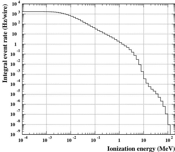
Fig. 7. Integral event rate at the centre of chamber.
