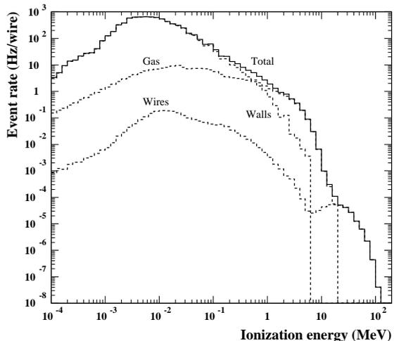
Fig. 5. Total event spectrum and its components at the center of chamber.
