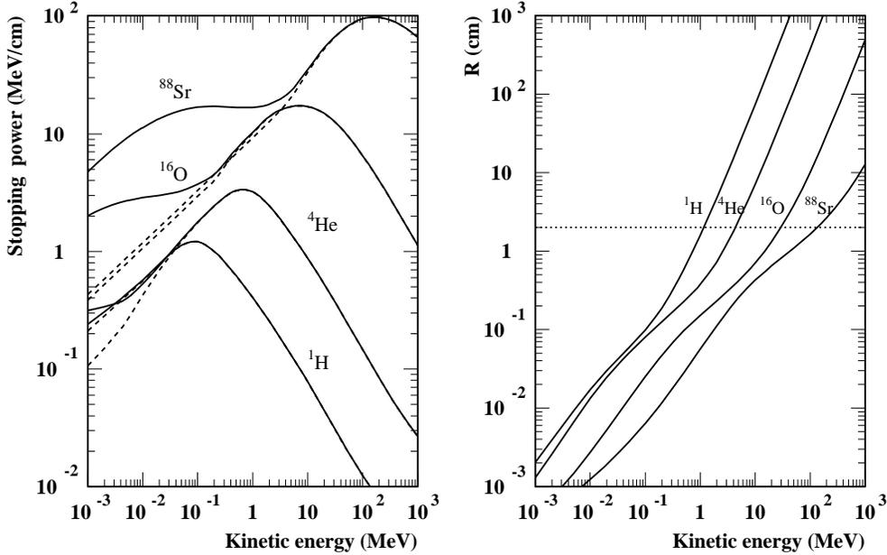
Fig. 2. Stopping powers (left) and ranges (right) of some ions in the ME1/1 gas. Dashed curves on the left figure represent the ionizing component of the total stopping power.
