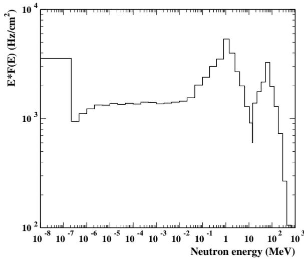
Fig. 1. Neutron energy spectrum in the ME1/1 chamber slot.
