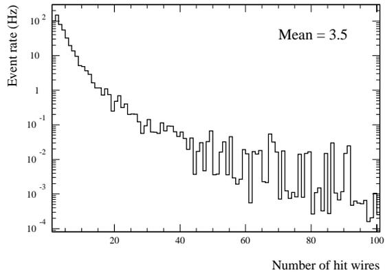
Fig. 4. Event rate distribution on the number of simultaneously hit wires.
