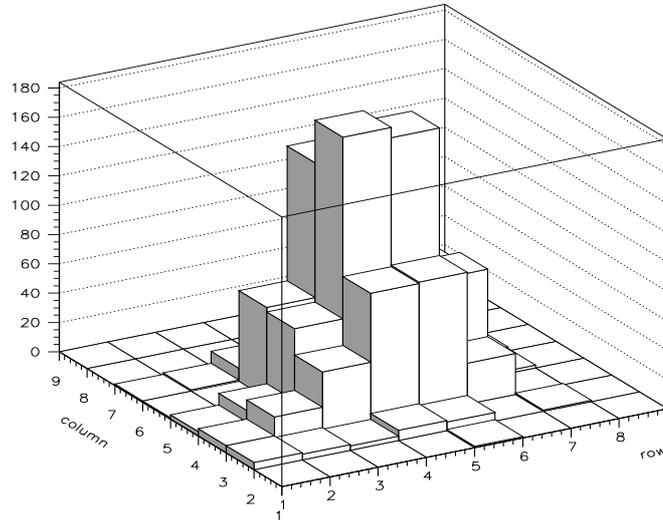
Figure 2. Population of  $8 \times 8$  matrix after  $\sim 1000$  cosmic triggers. HV=7.3 kV.
