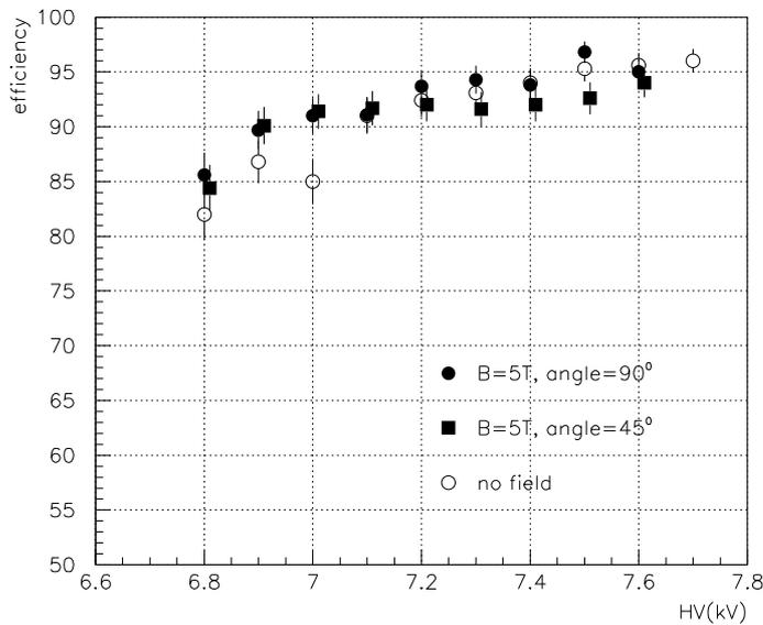
Figure 6. Efficiency as a function of HV.
