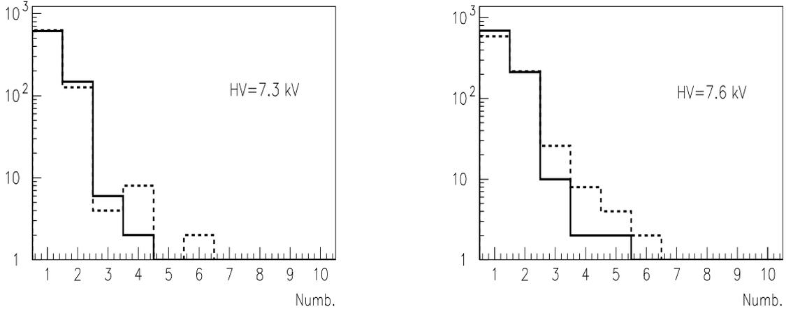
Figure 4. Multiplicity of the fired columns (solid) and rows (dashed) at  $HV=7.3 \text{ kV}$  and  $HV=7.6 \text{ kV}$ .
