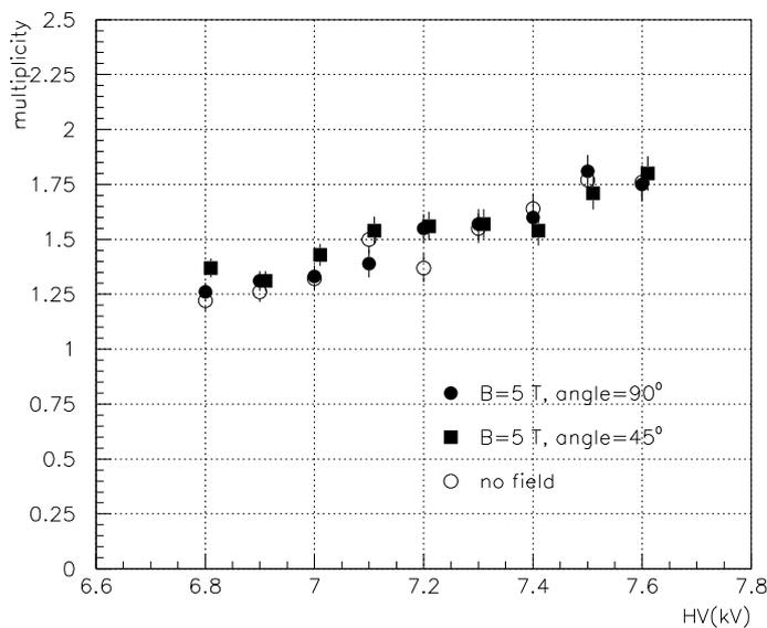
Figure 5. Multiplicity of the fired pads as a function of HV.
