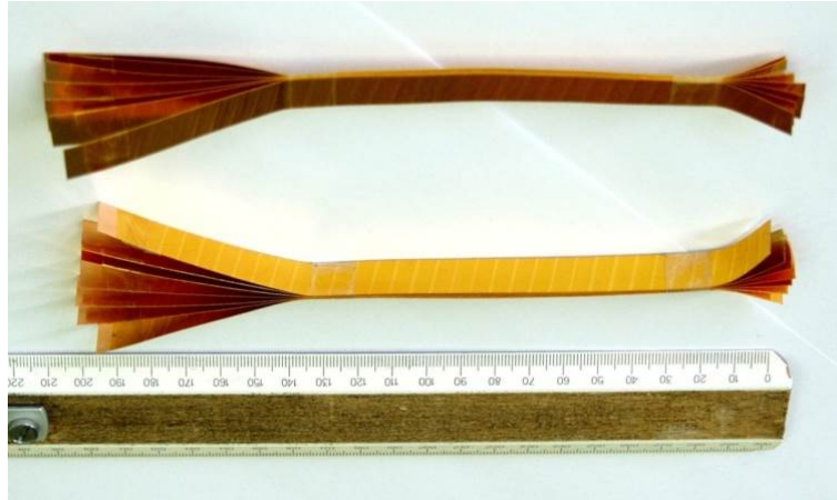
Figure 3. Stacks of insulated 2G HTS wires, used in electric strength measurements.
