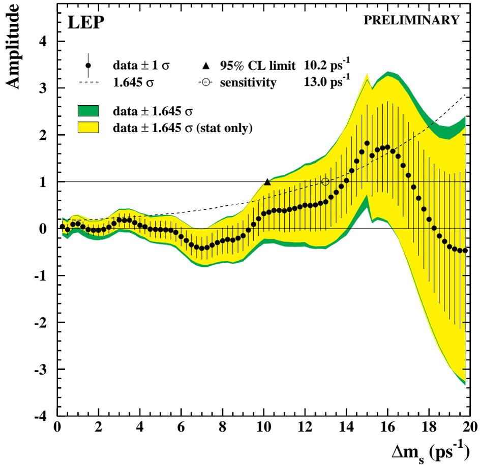
Figure 14: Lower limit on  $\Delta m_s$  as determined by the amplitude method.
