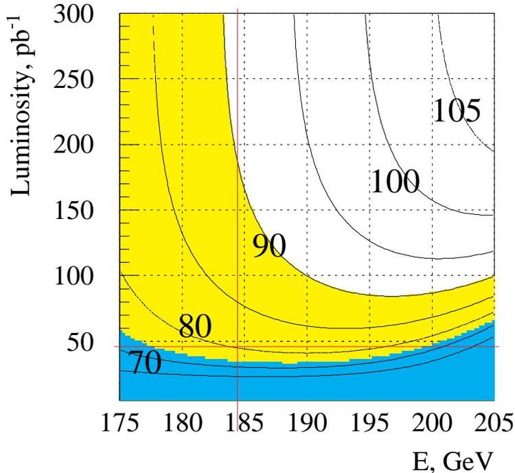
Figure 23: The luminosity per LEP experiment needed to discover a SM like Higgs boson, for various  $\sqrt{s}$  values.
