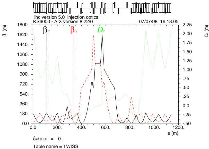
Figure 6:  $\beta$ -functions and dispersion around IP8 for a high- $\beta$  optics adapted to vertical and horizontal Roman pots taking into advantage of the low- $\beta$  triplet trim power supplies available in the standard design (10 %), from [18].
