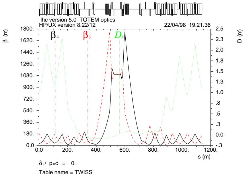
Figure 5:  $\beta$ -functions and dispersion around IP5 for the ideal high- $\beta$  optics adapted to vertical and horizontal Roman pots with low- $\beta$  triplet quadrupoles with three parameters, from [17].
